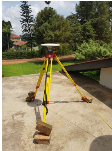
Figure 4.1: Measurement set-up for a dual frequency receiver at Ndejje Secondary School
