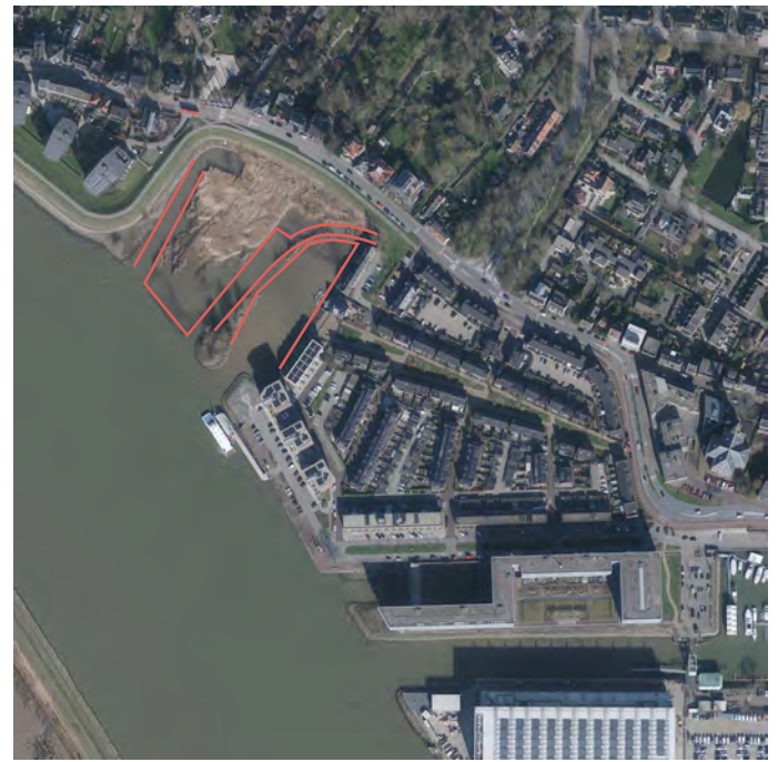
Figure 5. The shipyard of Smit in Alblasterdam in 1842 compared to today. The gantel, kielgat and berth can still be seen in today's landscape. Left image from De Ouwe Werf (p. 29), by B. Belder, 2005, De Stroombaan ; map made by J. M. van der Mall, 1842. Right image from "Beeldmateriaal Nederland," 2022 ( https://opendata.beeldmateriaal.nl/pages/downloaden ).
