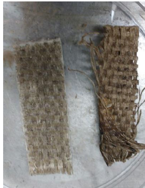
3.8 | Coated and uncoated samples tested for tensile strength after 808 hours in an QUV accelerated weathering machine
