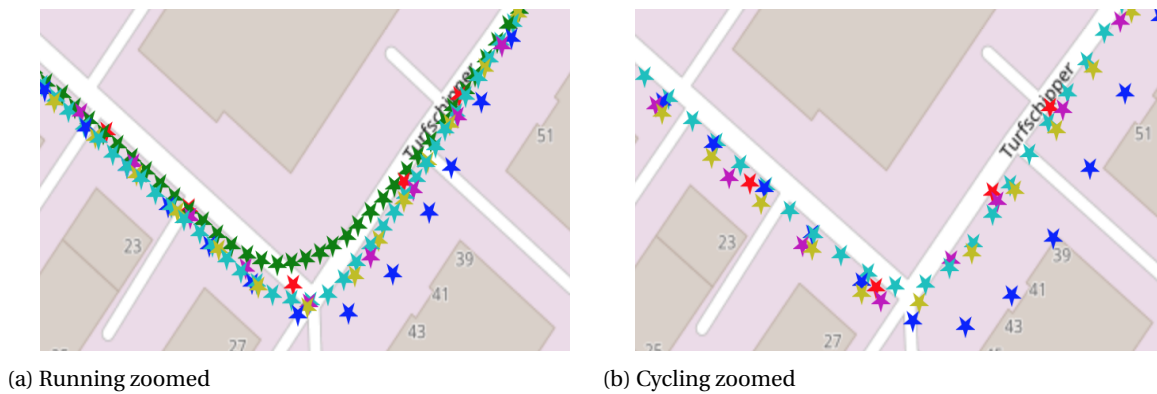
Figure 2.1: Same travelled path with approximately 15-16 km/h (running) and 26-27 km/h (cycling) using different apps. All paths were traversed on a bike to make it more easy to keep the speed constant. ● Endomondo, ● Fitbit, ● MapMyRun, ● Runkeeper, ● Runtastic, ● Strava
