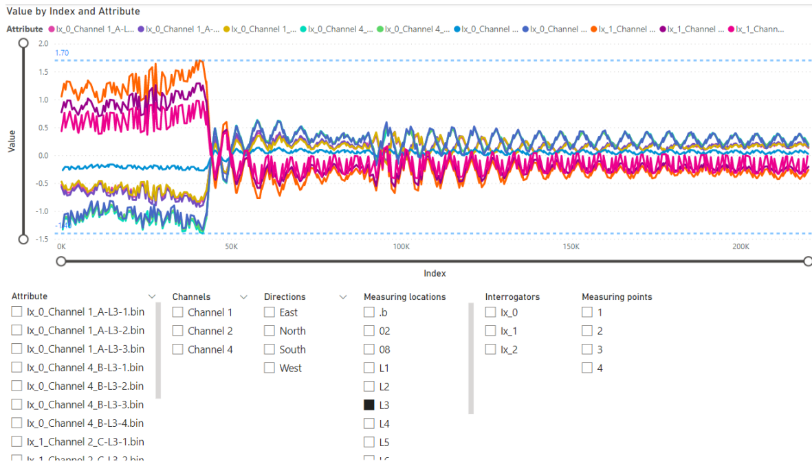
Figure A.19: Steel stress for L03 position
