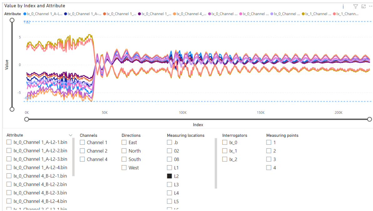
Figure A.18: Steel stress for L02 position
