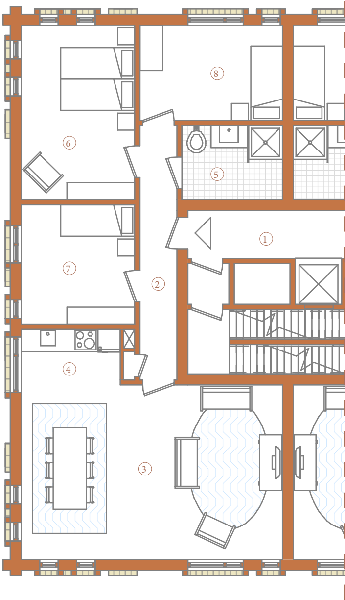
Figure 9.7 Typical Floor Plan 3-Bedroom Apartment in Tower [Scale 1:100]
