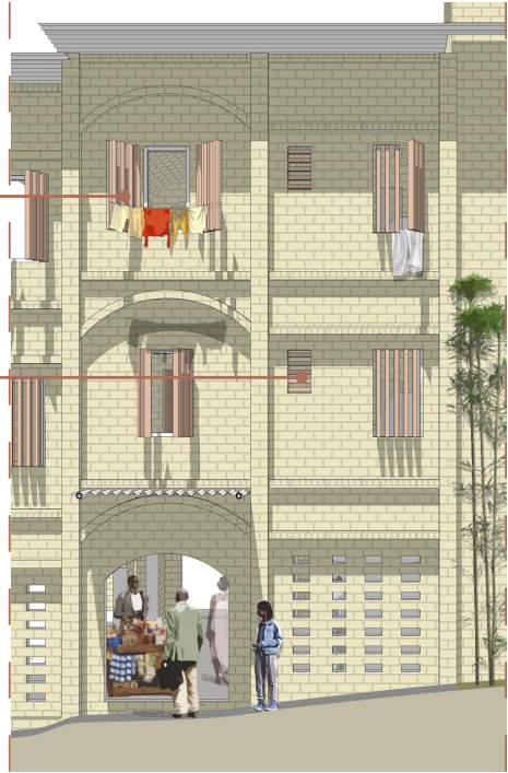
Figure 12.1 Manually Operatable Sun Shading at Retail Street
