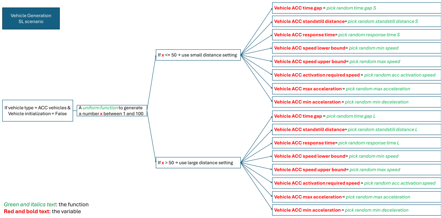
Figure 3.2: ACC vehicle generation process in VISSIM
