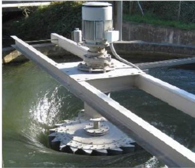
Figure 30: Gravitational water vortex turbine (Noortgaete et al, 2016)
