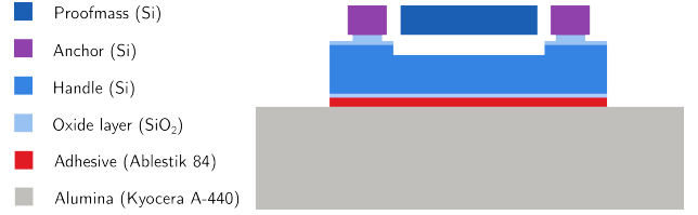
Fig. 5: A schematic illustration of the cross-section of the G6 accelerometer package showing the different layers that are bonded together (not to scale and thin metal layers not considered).
