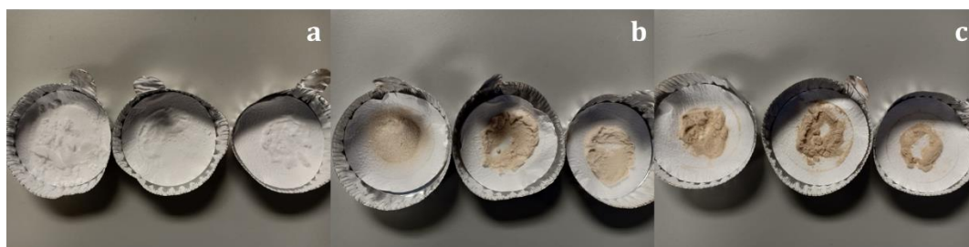
Figure 4.11 The colour of produced struvite crystals. a) 0 g TOC/L melanoidins, b) 0.5 g TOC/L melanoidins, and c) 1 g TOC/L melanoidins
