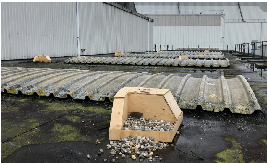
Figure 10 Forty prototypes of Nesting Hubs are being tested on the roof of an industrial warehouse during the 2024 breeding season. Source: J. van der Leun.
