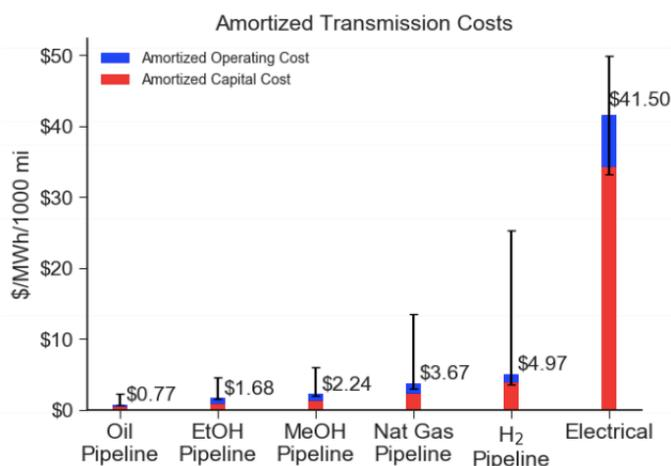
Figure 2.10: Amortized transmission costs comparison [29]
