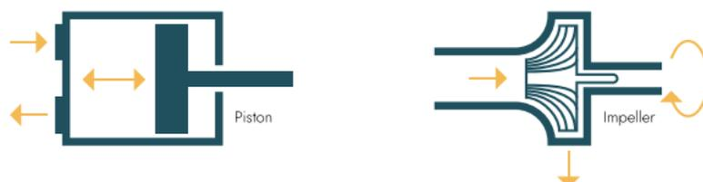
Figure 2.8: Schematic comparing reciprocating and centrifugal compressors, [54]
