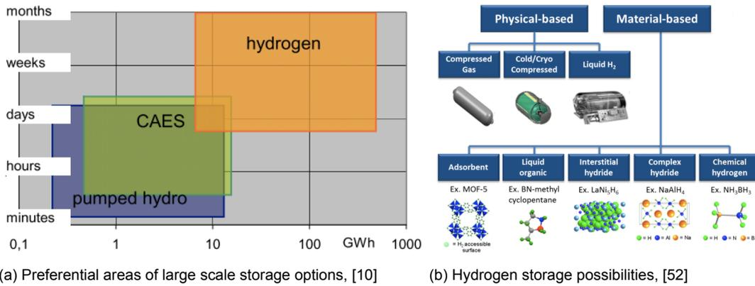
Figure 2.1: Hydrogen comparison with: other technologies (left) and storage possibilities (right)
