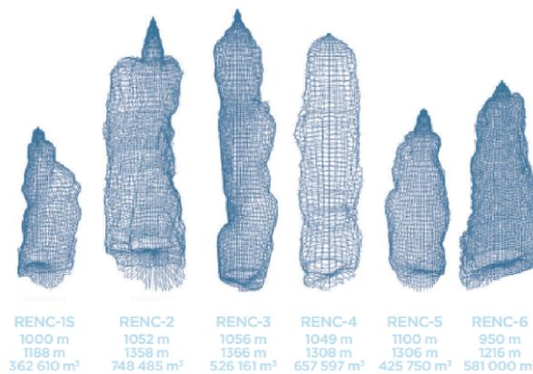
Figure 3.9: Schematic of the 6 Carriço salt caverns volume, [44]
