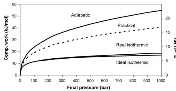
Figure 3.8: Energy required to compress hydrogen from 1 bar to the final pressure specified on the primary axis, [30]
