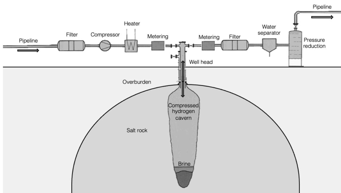
Figure 2.6: Storing process of hydrogen in salt caverns, adapted from [40] and [3]
