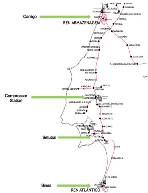
Figure 3.11: Partial map of natural gas network outlining important points, compressor station and relevant points [46]
