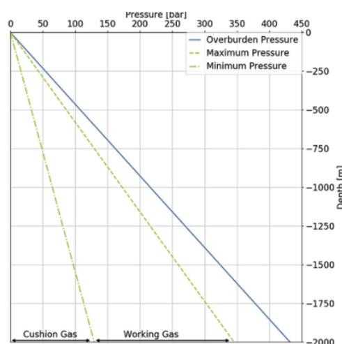
Figure 2.5: Estimated pressure limits as function of depth for hydrogen storage in salt caverns, [7]
