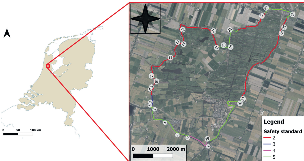
Figure 4.9 Left: map of the Netherlands, with the location of the Eilandspolder. Right: overview of levees protecting the Eilandspolder, the distinction into separate, numbered, levee sections, and their assigned flood protection standard.
