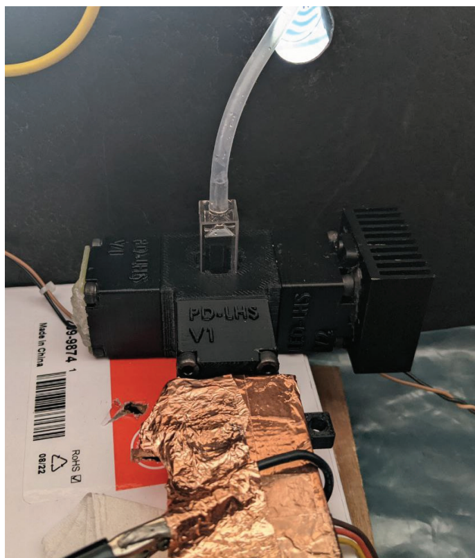
Testing the flowcell in PRI's optical engine testing setup to determine if it would effect its output.
