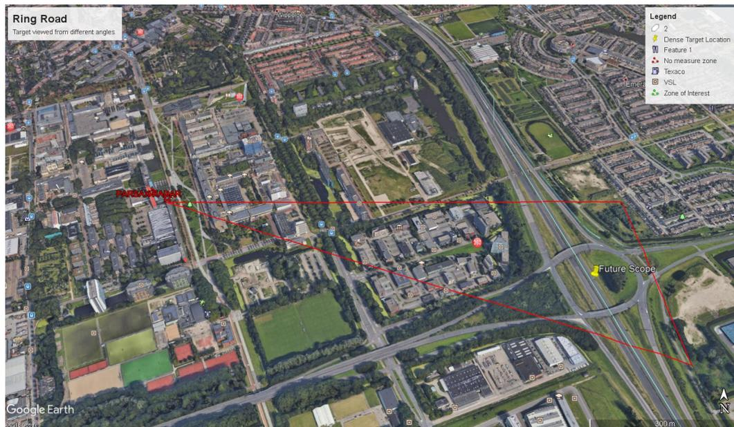
Figure 7.2: Round About on N470 highway, targets moving will provide returns at different angles, due to the turns around the round about
