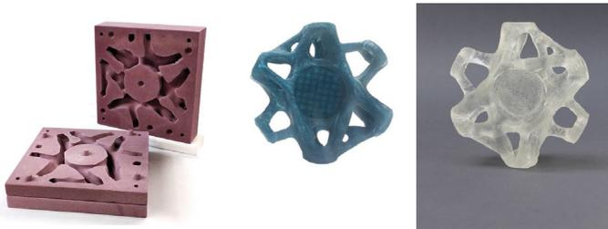
Fig.8: Left: 3D-printed sand moulds produced by ExOne; middle: 3D-printed wax positive model. right: cast glass prototype of the grid-shell node made by the wax model and a silica-plaster mould
