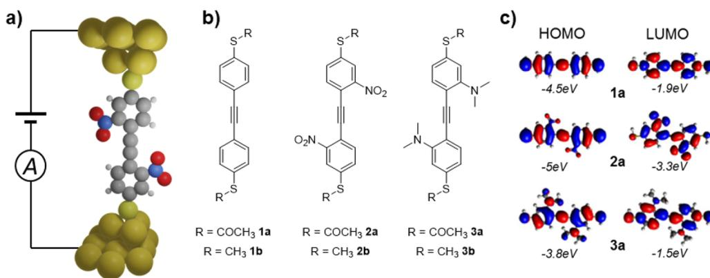
**Figure 1.** Schematic of molecular junctions formed. (a) An example of a tolane molecule with a nitro substituent and thiol anchor group connected to two gold electrodes; (b) the series 1–3 of tolane model compounds with acetyl masked thiol anchor groups (a) and methylsulfide anchor groups (b); (c) frontier molecular orbitals of 1a, 2a, 3a.
