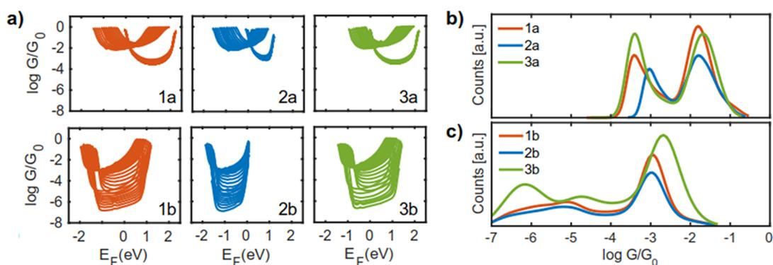
**Figure 5.** Calculated conductance histograms. (a) Conductance for molecule 1, 2, and 3 with different anchor groups and contacting conformation to electrodes; conductance histograms based on conductances in (a) for a wide range of Fermi energies between the HOMO–LUMO gap for 1a, 2a, and 3a (b) and for 1b, 2b, and 3b (c).
