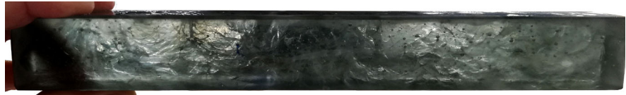
Fig. 7 “Lead CRT, 870 °C” specimen containing intense cord (seen as wavy lines) and bubbles
