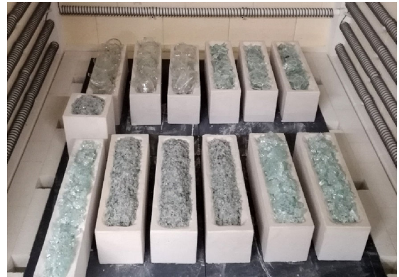
Fig. 1 Arrangement of the investment moulds inside the ROHDE ELS 1000S kiln
