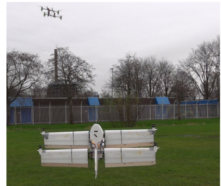
(c) Separate flight; Both aircraft are in attitude control.
