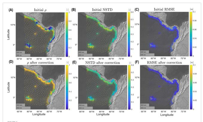
Goodness-of-fit statistics at the computational nodes by employing the optimized model (test run 10, bulk correction): (A)  $\rho$  before correction, (B)  $\sigma$  before correction, (C) *RMSE* before correction, (D)  $\rho$  after correction, (E) *NSTD* after correction, and (F) *RMSE* after correction.
