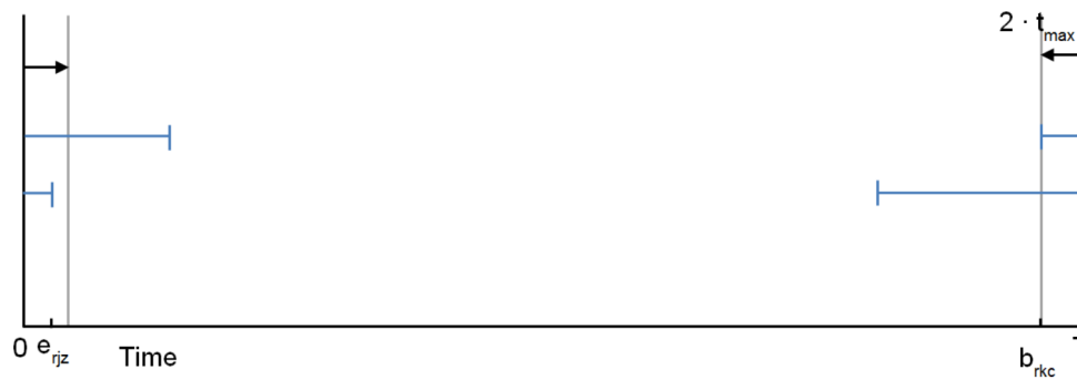
Figure 4.7: Graphical representation of the begin time of a cancelled train being between 0 and t_{max} , and the corresponding time window in which the end time of another route needs to lie in so that time shifts lead to a prevention of overlap of blocking times at a resource.
