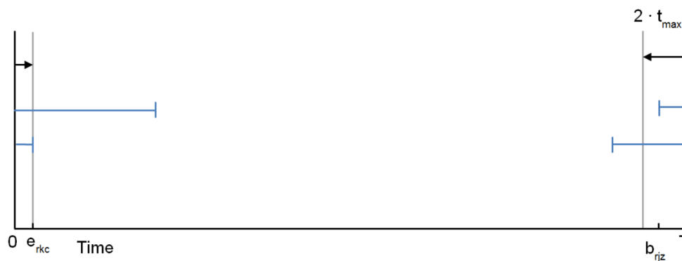
Figure 4.8: Graphical representation of the end time of a cancelled train being between 3599 - t_{max} and 3599, and the corresponding time window in which the begin time of another route needs to lie in so that time shifts lead to a prevention of overlap of blocking times at a resource
