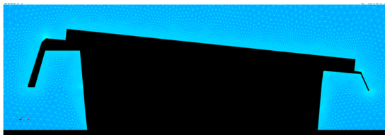
(a) Zoomed in view of the geometry and mesh of the FPV used in literature.
