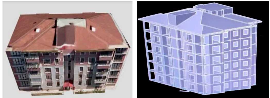
Figure 5. The photogrammetric (left) and architectural (right) model of a 3D building produced by GDLRC, adapted from [56].
