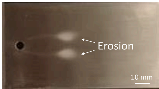
Fig. 16. (Top view of the sample plate) Mass loss (erosion) pattern on stainless steel at a flow velocity of 50 m/s ( Re = 2.5 \times 10^5 ).
