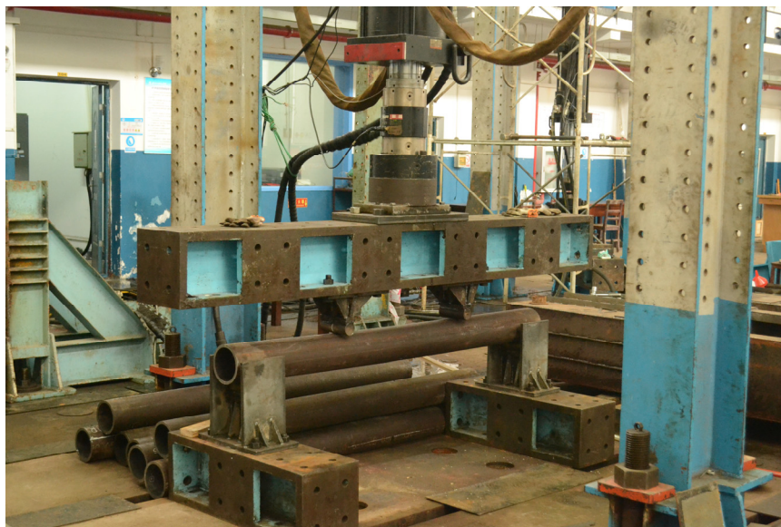
Figure 3.14. Four-point bending test set-up: the schematic and specimen configuration is shown in the upside; actual test set-up is shown in the downside
