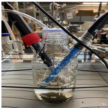
Figure 2.2: Experimental setup of the anoxic batch reactor
