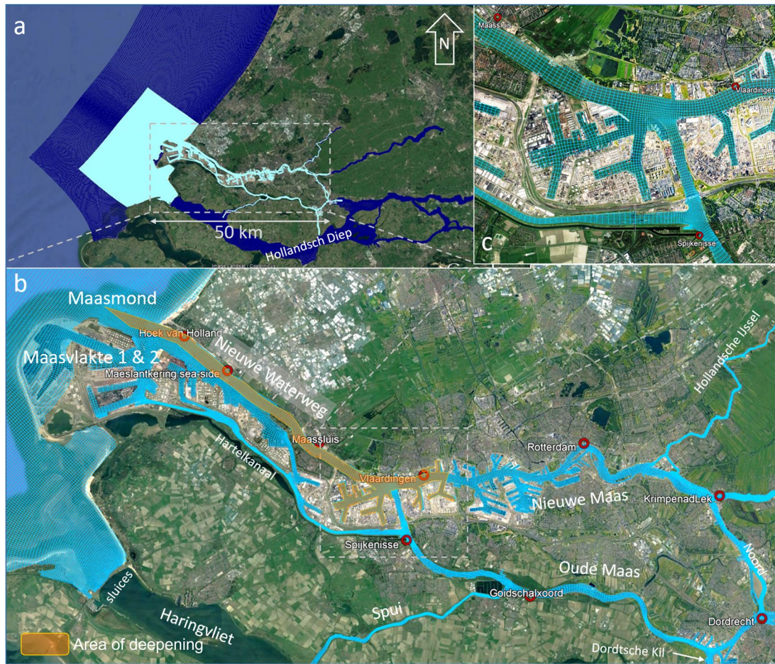
Figure 1. Aerial photographs of the Rhine-Meuse Delta, along with the model domain and names of the branches. (a) Model domain. The dark blue area indicates the larger 2D-model from which the smaller 3D-model (light blue) derives its boundary conditions. Both domains have the same grid size. (b) Model grid of the smaller 3D-model with red circles indicating the locations of measurement stations that were used for model validation. (c) Inset of the model grid at the bifurcation from the Nieuwe Waterweg (West) to the Nieuwe Maas (East) and the Oude Maas (South).
