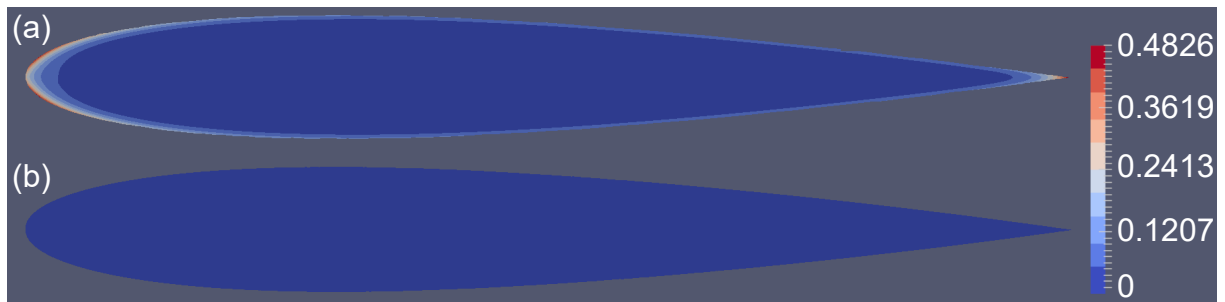
Figure 2: Flow past NACA0012 at Re=1000 modelled using (a) penalty forcing method and (b) domain decomposed method. The figure shows the magnitude of non-dimensionalised velocity inside the solid domain.
