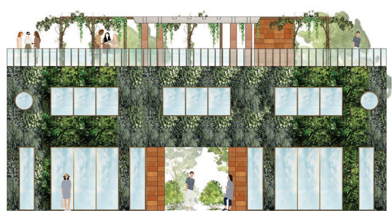
Facade 3: Green facade and replacement of windows
