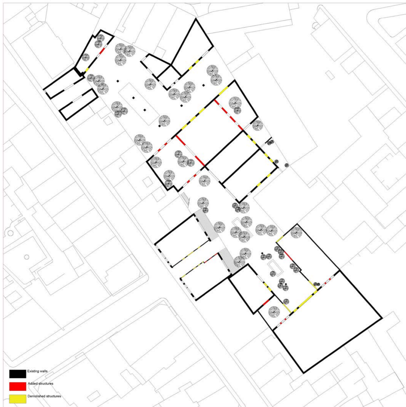
Figure 52: Site plan. Drawing illustrates what was demolished and added to the existing site plan in order to design alternative proposition.
