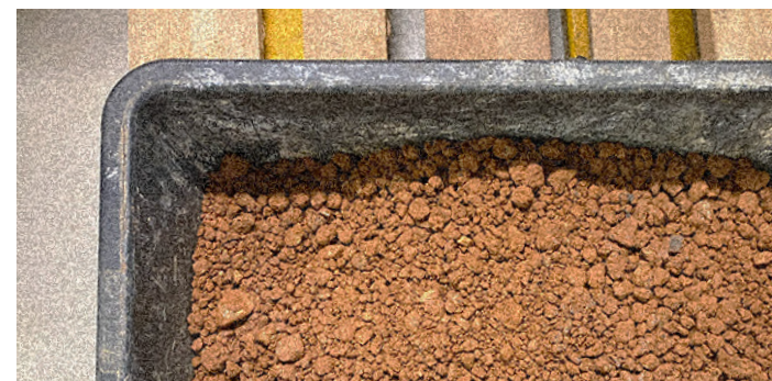
Rammed earth mixture.
