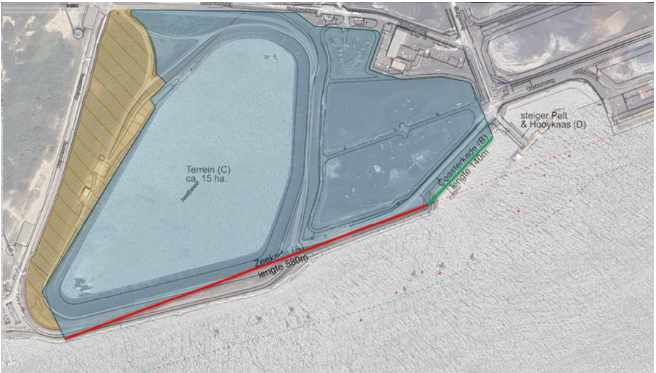
Figure 3 Proposed location of the quay wall. A (red colour) indicates the deep sea quay and B (green colour) indicates the coaster quay (Port of Amsterdam, 2023).
