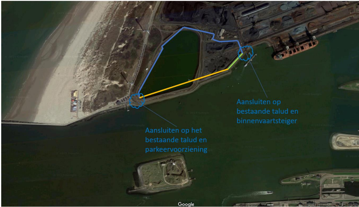
Figure 36 The quay wall and terminal area with the connection interfaces indicated (Witteveen + Bos, 2021).
