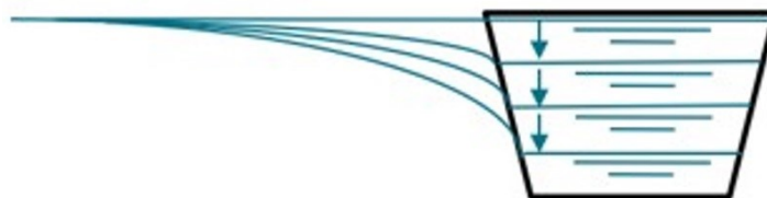
Figure 3.4: Local groundwater level lowering D2loc
