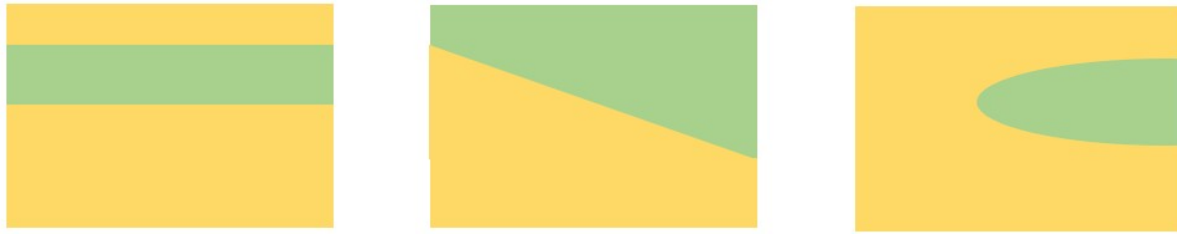
Left: horizontally oriented layers (SS1), Middle: inclined oriented layers (SS2), Right: weak spot (SS3), Green: weak soil, Yellow: strong soil
