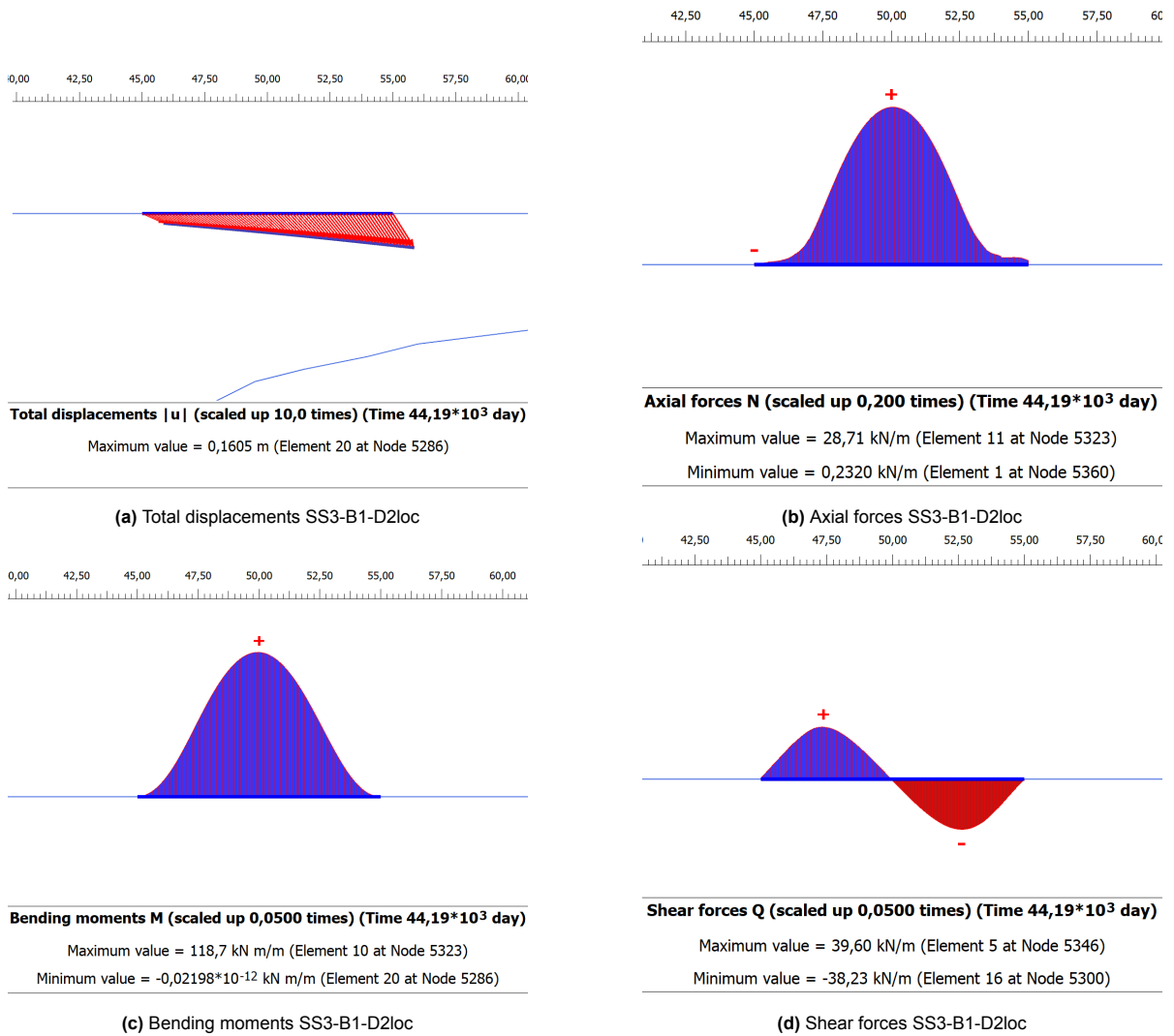
Figure 4.40: Internal forces and total displacements for scenario SS3-B1-D2loc
