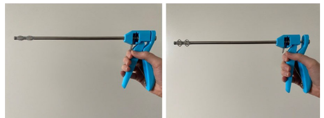
FIGURE 5. Prototype of the drill guide. Left: non-activated state; Right: activated state.
