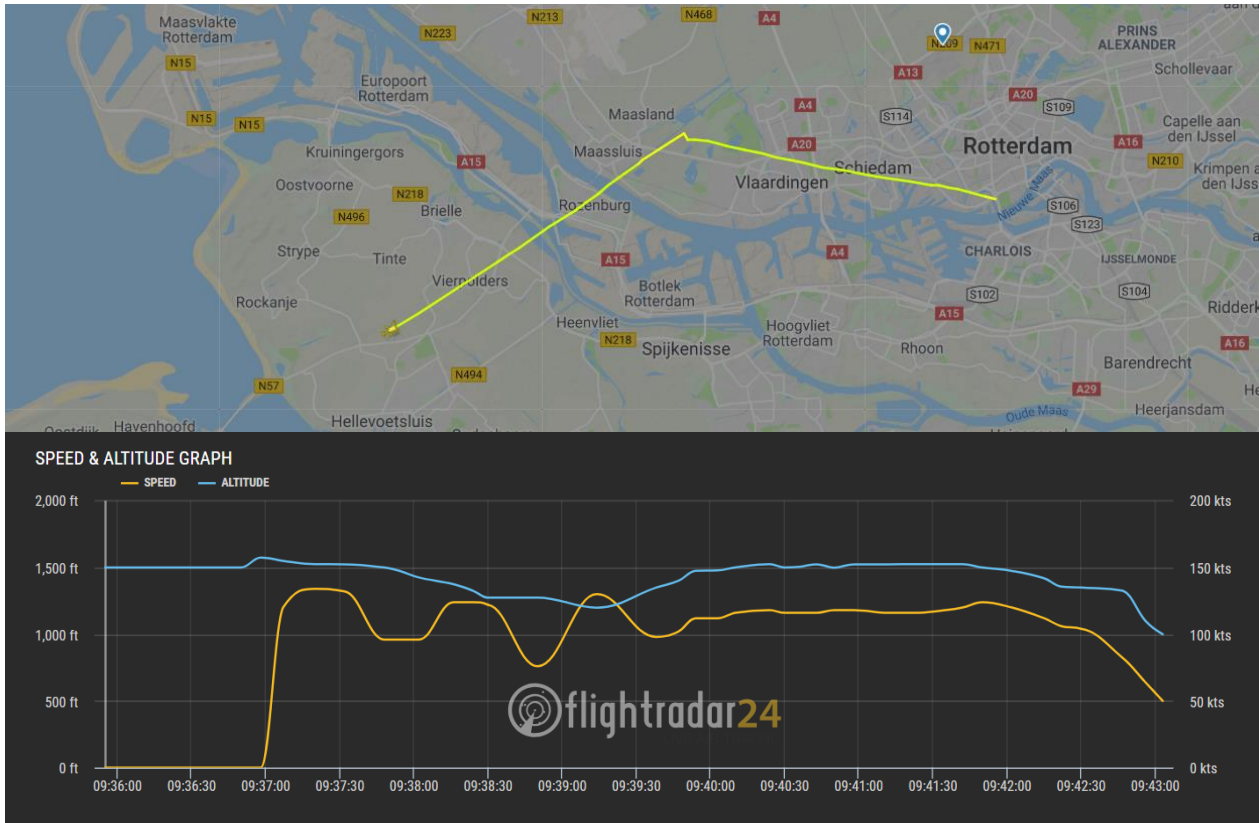
Figure 35: PH-HVB flight from a field to the nearby Rotterdam university hospital, 24 th April 2019 [50], showing the very low altitude generally flown by emergency response helicopters.
