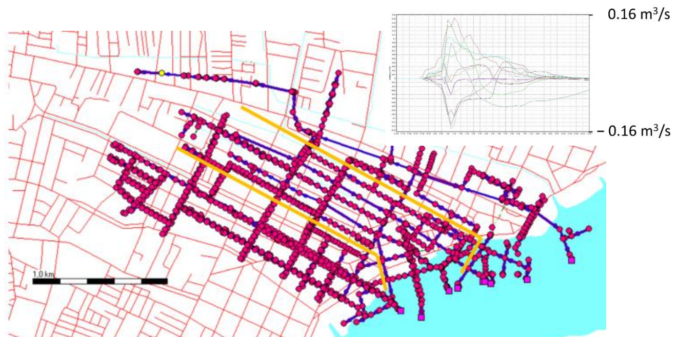
Figure 3-12 Schematisation of SOBEK 1D model. Yellow lines show the boundary of the catchment area. The graph displays all the in and outflows at the boundaries for a T=100 event are low and level each other out.
