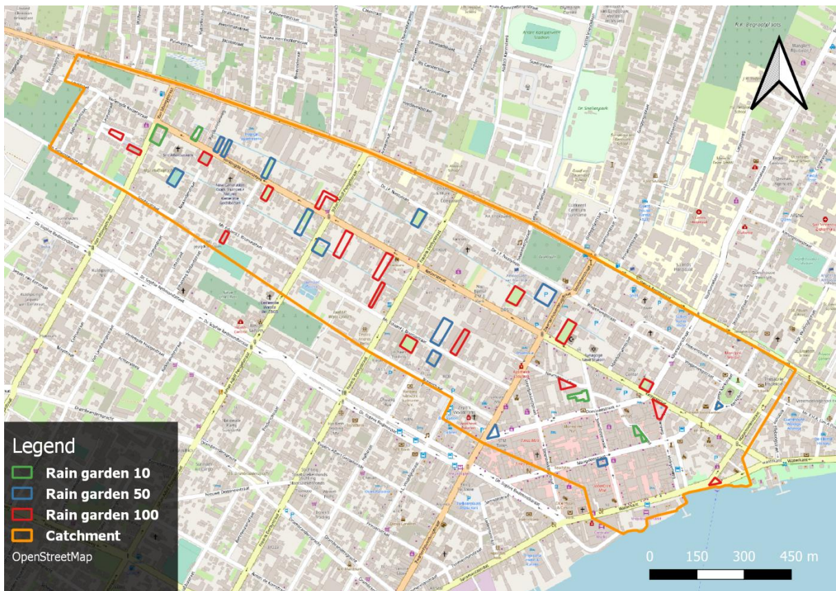
Figure 4-4 Study area with potential areas for Rain garden/Retention ponds. Green + blue + red represent maximum (100%) implementation, Blue + green represent realistic (50%) implementation and Green represents local measures only (10%).
