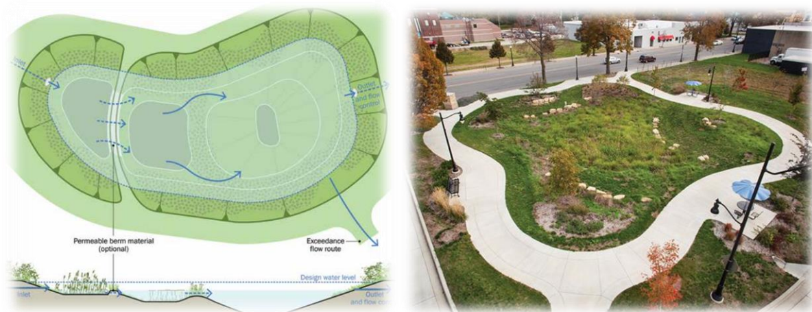
Figure 2-7 Concept of retention (left) and example of detention basin (right) (Woods Ballard et al., 2015)
