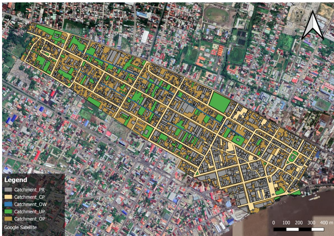
Figure 4-1 Land use area types divided according to the classification of the CRCTool. PR = Paved Roof, CP = Closed Paved, OW = Open Water, UP = Unpaved and OP = Open Paved.
