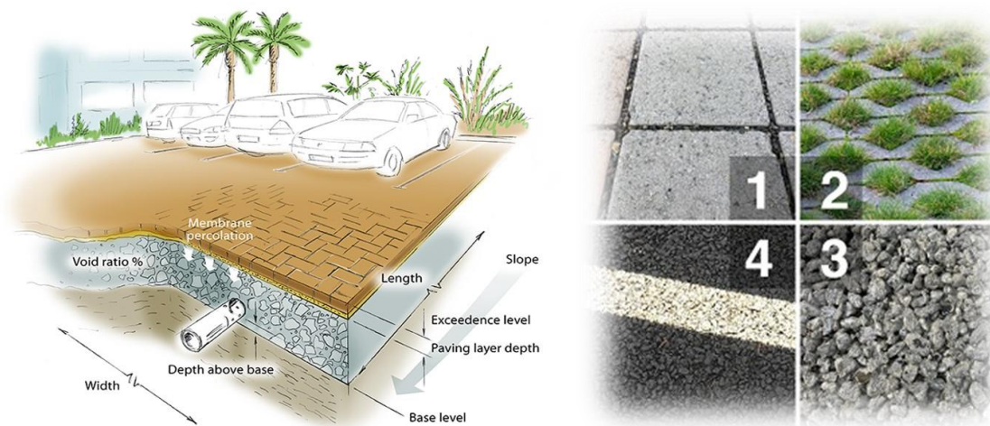
Figure 2-5 Permeable pavement concept and different pavement types: 1: permeable pavers, 2: grass pavers, 3: permeable concrete, 4: permeable asphalt (Ellis R, 2018)
