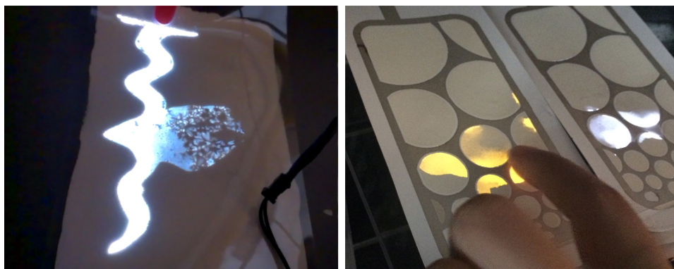
Figure 4.2 – Using water as a replacement for the printed conductor: the bottom-emitting sample (left), top-emitting sample (right).
