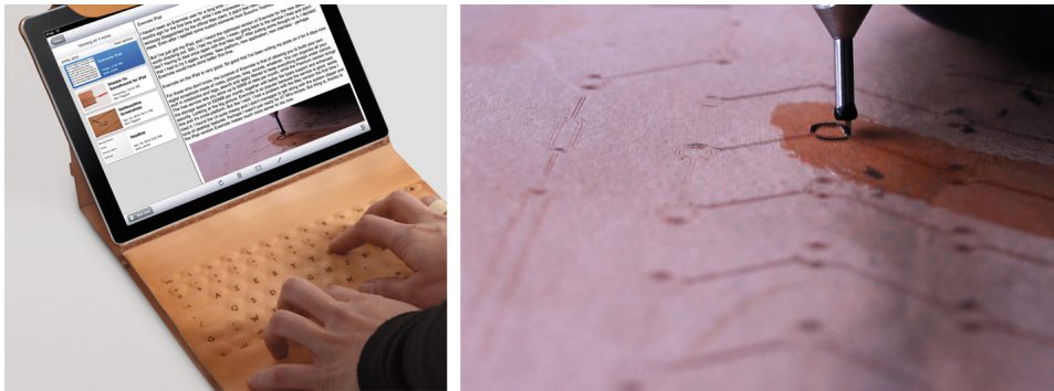
Figure 5.5 – A novel potential of the leather has been unlocked in relation and through the skillful act of tattooing the conductive ink.
