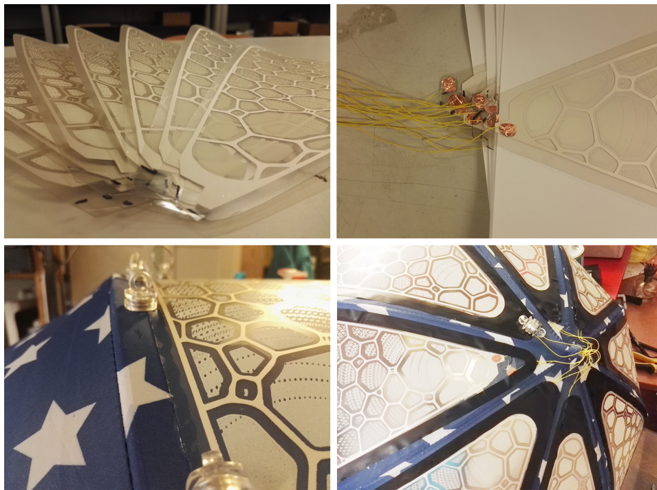
Figure 3.15 – Integration process of the EL sheets in the final prototype: eight water-activated EL sheets (top-left), preparing the connections (top-right), juxtaposing the EL sheets (bottom-left), wiring through the shank (bottom-right).
