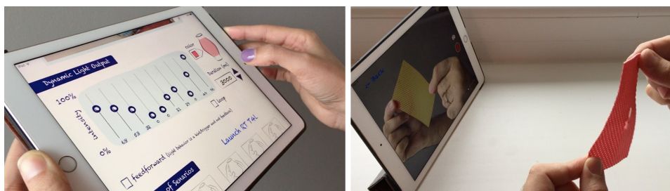
Figure 2.13 – The real-time Chroma-key app: a snapshot of the interface (left), the user can select the color by touching it on the screen and use the slider to fine-tune the threshold (right).
