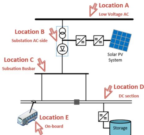
Fig. 5: Different PV and ESS placement possibilities
