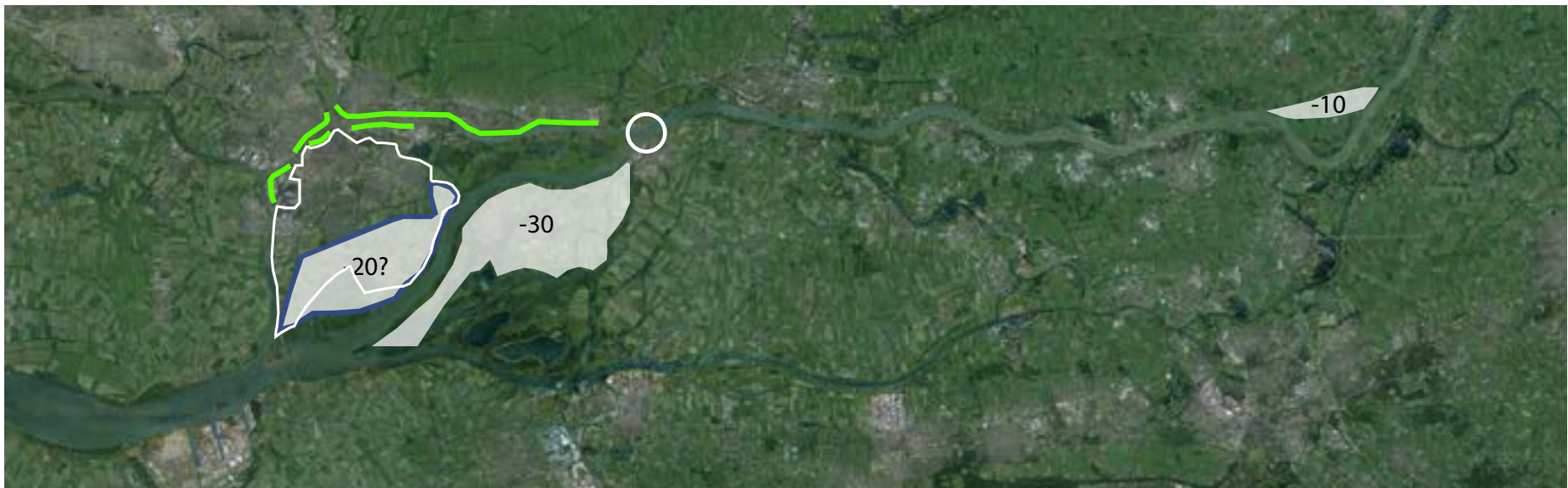
Figure 28. Room for the River type of intervention could lower water levels by 20cm for the entire waterfront of the Drechtsteden.
