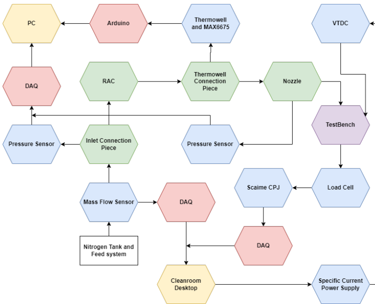
Figure 6.6: Schematic of the experimental hardware
