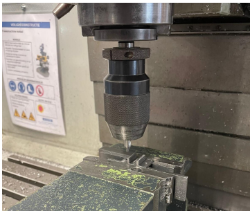
(a) Nozzle support manufacturing in the milling
