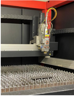
(a) Laser cutting machine used for the support's base
