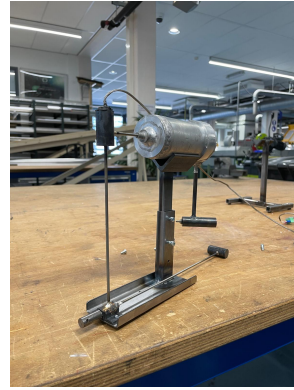
(b) Thruster support assembled
