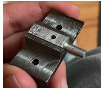
(b) Nozzle and its support before welding
