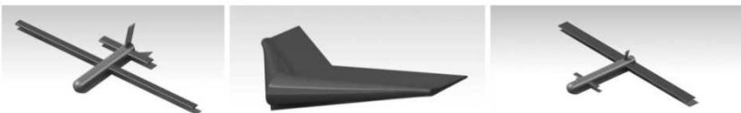
Figure 6.1: the three main UAV design concepts. From left to right: standard horizontal tail configuration, flying wing and canard configuration.
