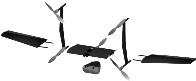
Figure 15.2: Tail sitter showing its main components and assembly points
