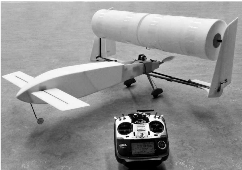
Figure 23.7: Remote controlled Magnus Aeolus Model
