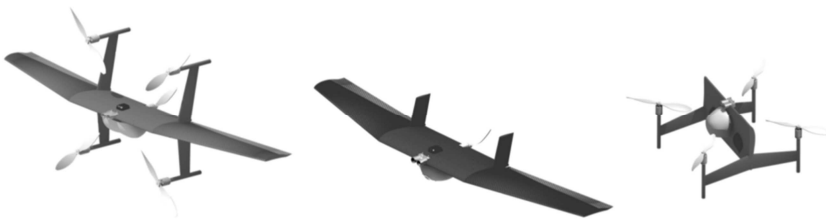
Figure 15.1: The three configurations of MIRU (f.l.t.r.): a tail sitter, flying wing, and quadcopter
