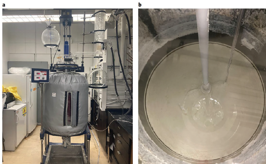
Figure 10. a) Photo of a kg-scale synthesis of MOF-303(Al) in a 200 L reaction vessel, and b) formation of slurry after refluxing for 6 h. Reproduced with permission. [88] Copyright 2022, Springer Nature.
