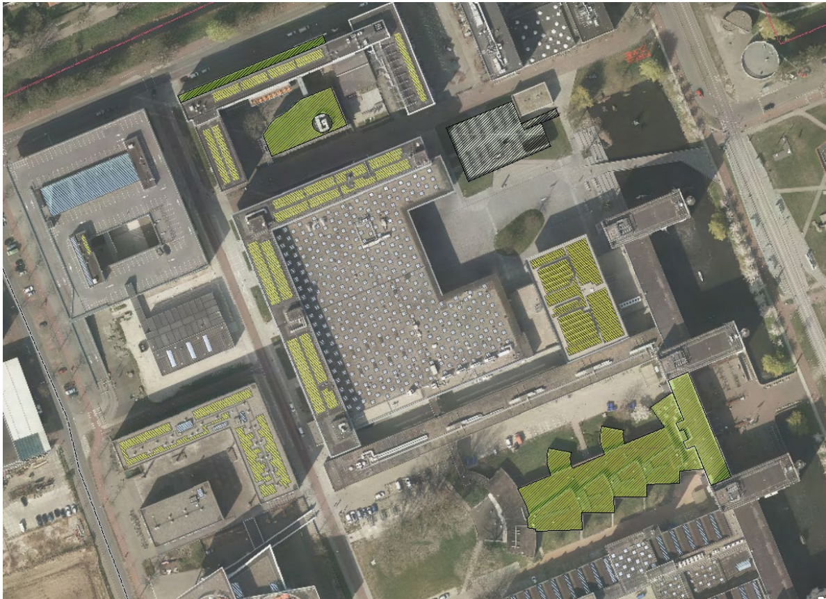
Figure 15: Existing PV arrays, green roofs and rooftops covering the TPM, ID and 3mE buildings
