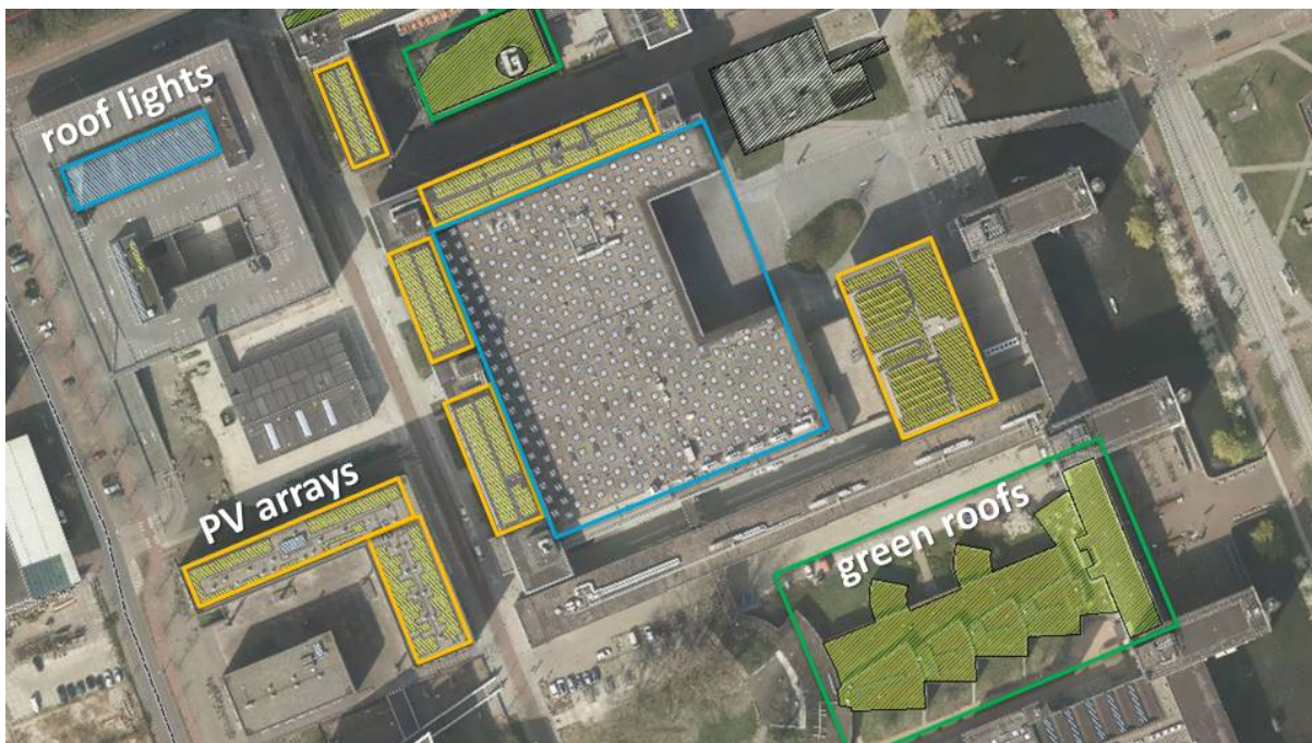
Figure 7: example of existing roof uses: green denotes green roofs, yellow PV arrays, blue denotes roof lights. More on this map at paragraph 4.1.
