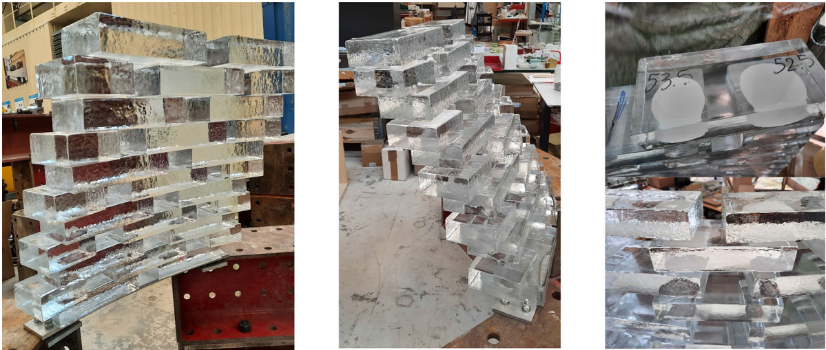
Fig. 13 Prototype constructed at the TU Delft Glasslab, showing the natural tilt of the bricks due to the larger cantilevering width in the initial design (left and center). The application of the Fast-Curing Experimental Adhesive in blobs may be visible from top view (top right), but cannot be easily seen from the side view (bottom right), and is thus not obstructive
