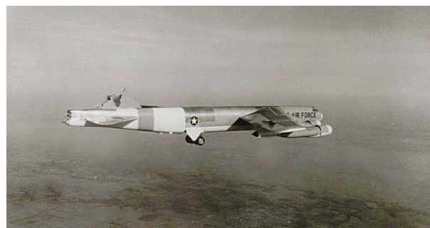
Figure 2.1: A Boeing B-52 having lost the majority of its vertical tail due to wind shear. The aircraft successfully landed, was restored and flew again. The aircraft remained in service with the USAF until 2008.
