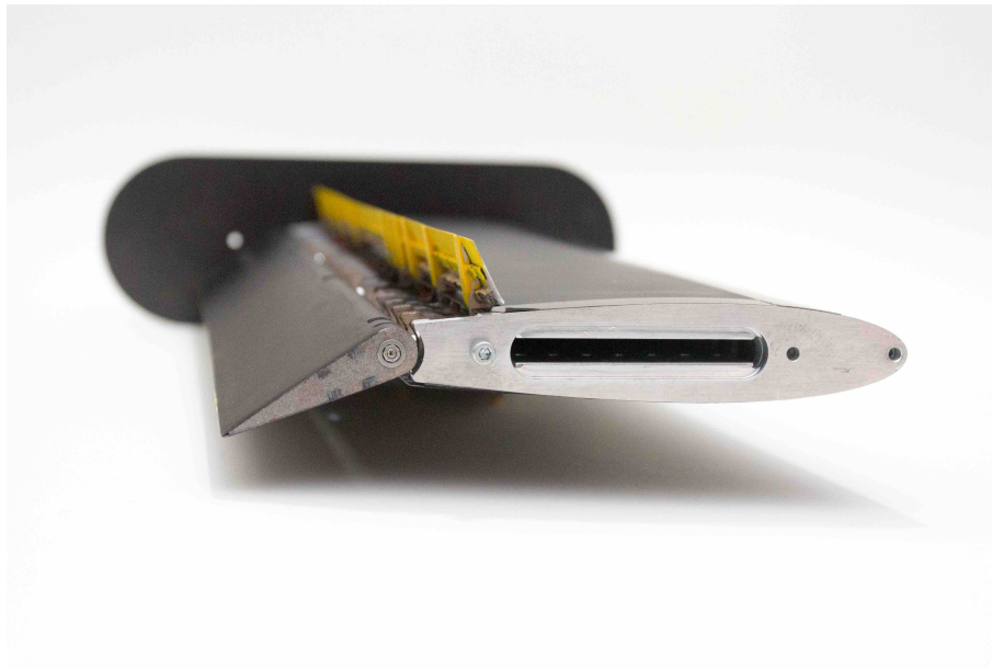
Figure 4.24: Side view of the wing section with the spoiler and aileron deflected. The right endplate is removed in this picture.
