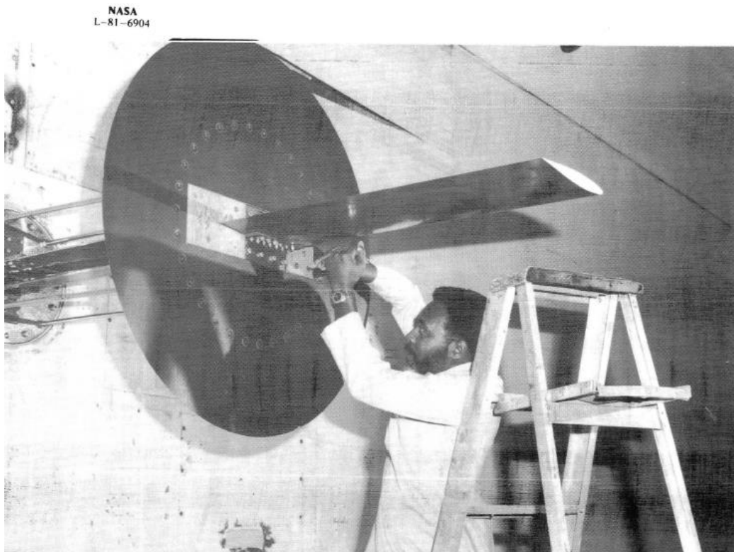
Figure 7 A wing installed on the mount system in the wind tunnel [1]
