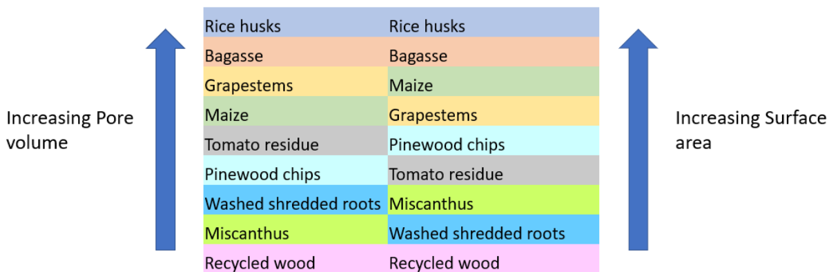
Figure 4.53: Biochar ranked in decreasing order for surface area and pore volume
