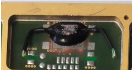
(a) Resistor attachment to the LO board.
