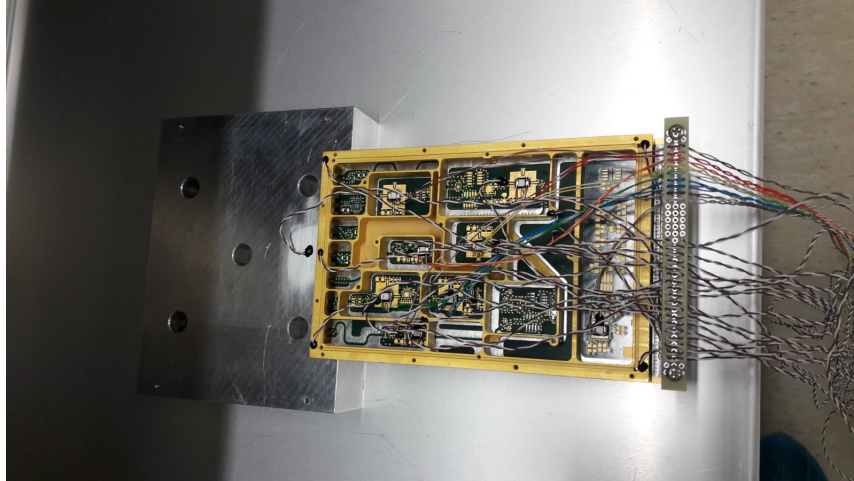
Figure 5.20: The test setup for the 2-4 GHz board.
