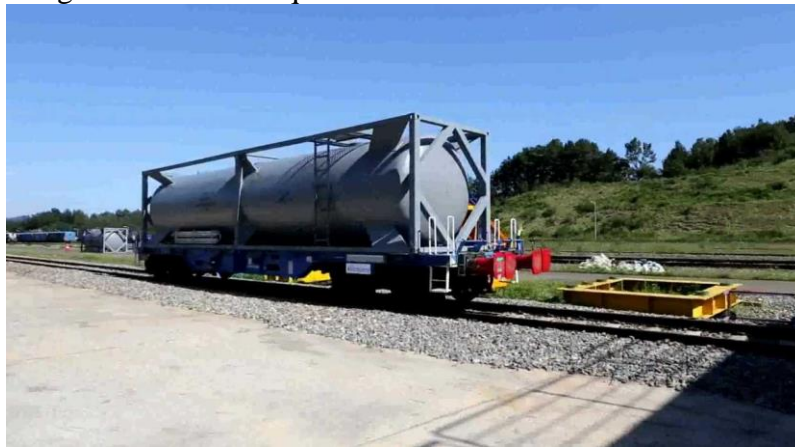
Figure 6- 10 Transportation of tank container by gondola car (normal loading)
