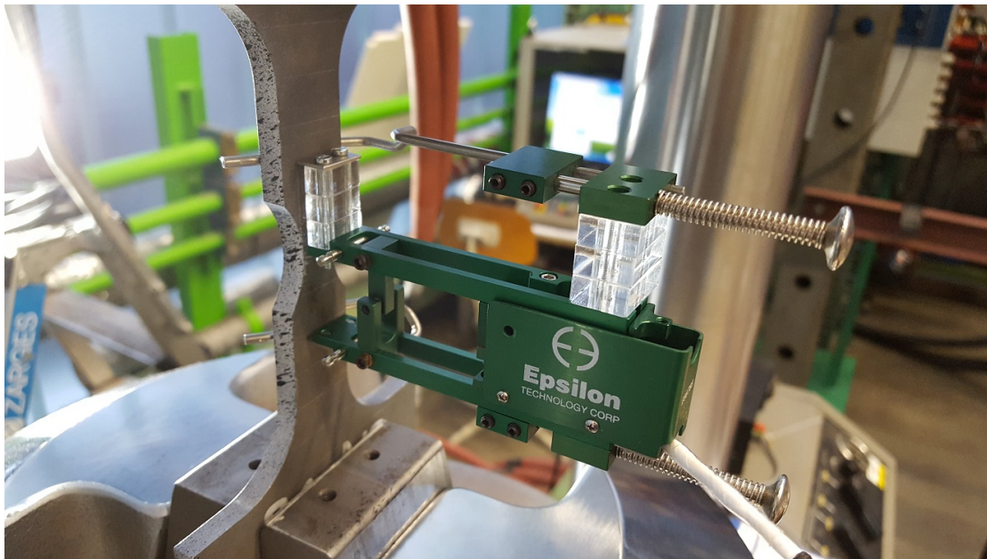
Figure F.1: Modified Epsilon 3542-025M-050-LT extensometer mounted on notched tensile specimen R1N1
