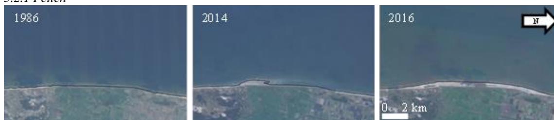
Figure 7 Time-lapse of the SDW position detected on a composite image of 1986 (left panel), 2014 (middle panel) and 2016 (right panel).
